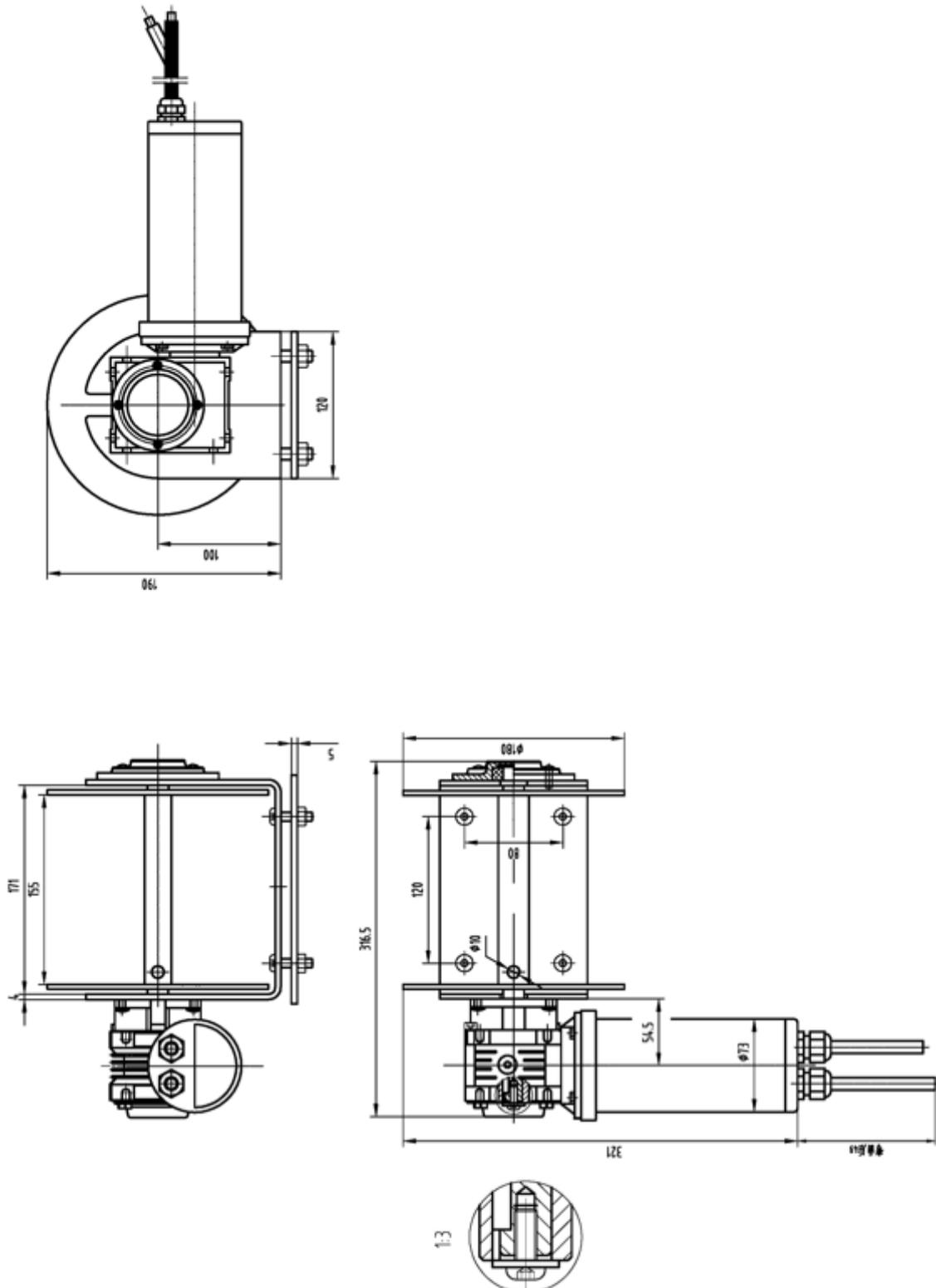
Dimensional Drawings for Savwinch 450CS/SS
