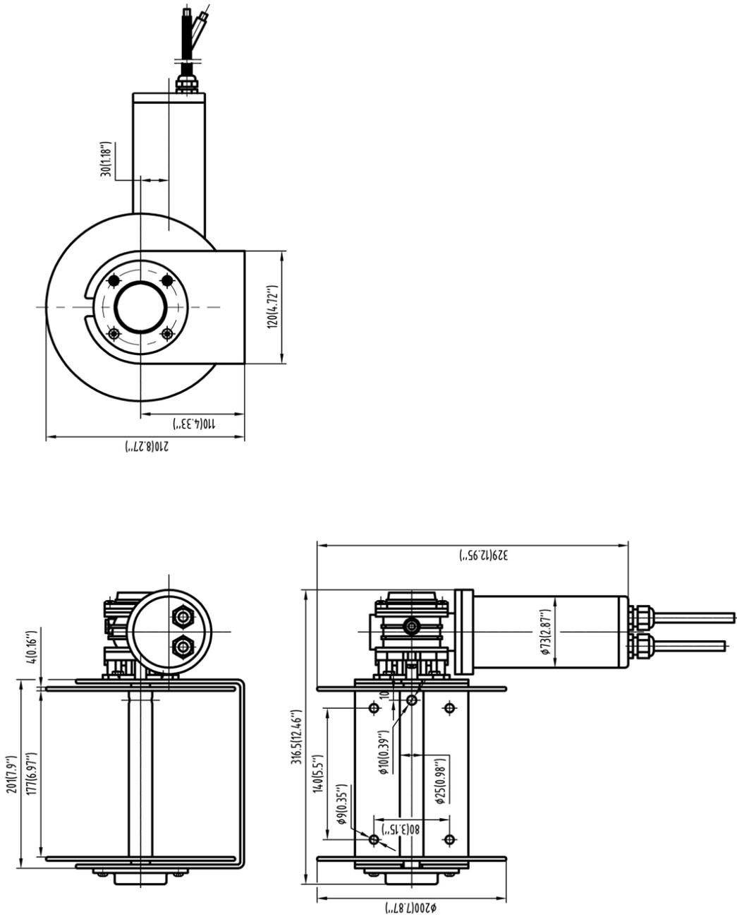
Dimensional Drawings for Savwinch 880CS/SS
